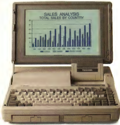
TI600: 11.6 lbs, Battery-powered 12MHz 286, 20MB hard disk, 1.44MB floppy, 1MB RAM expands to 5MB, backlit EGA LCD, removable/rechargeable battery packs.
